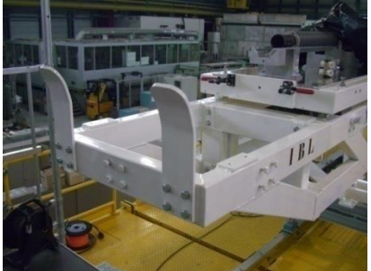
Pit Table extension: Removed during lowering put back in place after rotation
