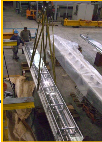
Pit Table extension: Removed during lowering put back in place after rotation
