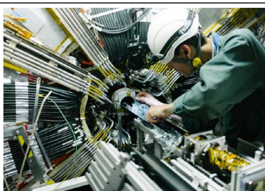
Beam pipe is pulled out in its transport container
