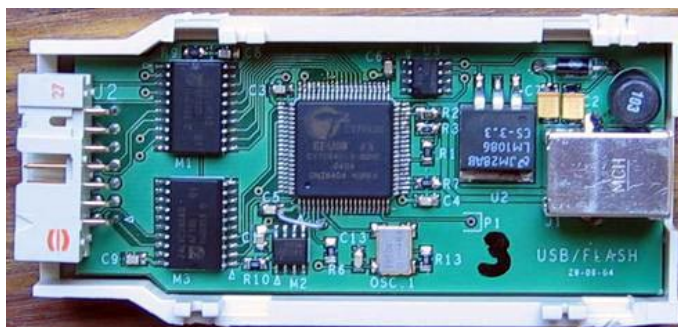
Figure 10: Carte Interface USB-GPIB.
