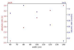
Fig. 4. Capture rate on  $^{238}$ U in the fertile salt depending on fertile blanket width.
