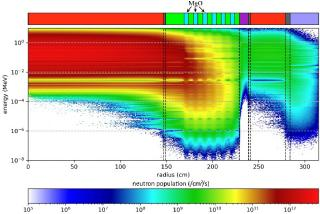
Fig. 6. Neutron spectrum with layers of moderator for Cl-MSFR
