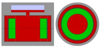
Fig. 3.: Model (Serpent2) of the fuel circuit for transport codes Legend: fuel salt in red; fertile salt in green; protection/envelope in dark grey; structure in grey; inert gas in light purple.
