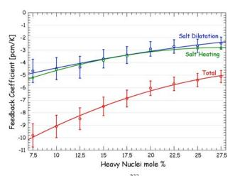
Fig.6. Feedback Coefficients of <sup>233</sup>U-started TMSRs at equilibrium as a function of the HN proportion
