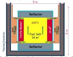
Fig.2. To scale vertical representation of the TMSR, including pumps and heat exchangers (IHX)
