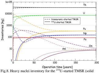
Fig.8. Heavy nuclei inventory for the <sup>233</sup>U-started TMSR (solid lines) and for the transuranic-started TMSR (dashed lines) with 17.5 mole% of heavy nuclei in the salt
