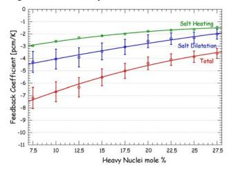
Fig.7. Feedback Coefficients of Pu-started TMSRs after one year of operation as a function of the HN proportion
