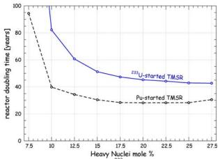
Fig.10. Reactor doubling time of  $^{233}$ U-started (solid line) and Pu-started TMSRs (dashed line) for different HN proportion configurations and with a reprocessing of 200 kg / day
