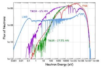
Fig.5. Neutron spectrum of two TMSR configurations (6% and 27.5% of heavy nuclei in the salt) compared to the neutron spectrum in a Light Water cooled Reactor (LWR) and in a Fast Neutron Reactor (FNR)
