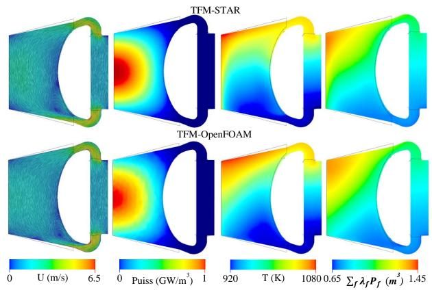
Figure 4 - Comparison between TFM-STAR (top) and TFM-OpenFOAM (bottom) of velocity field, power field, temperature field and precursors decays field at steady state
