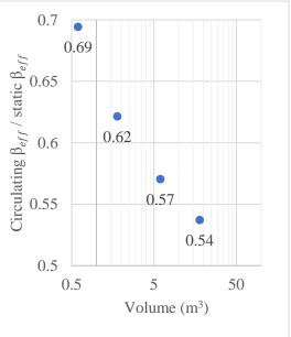
Figure 12 - Evolution ratio between the circulating and the static  $\beta_{eff}$  as a function of the reactor size
