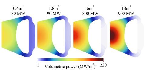
Figure 10 - Volumetric power for different core sizes (0.6m3 to 18m3) and various levels of power
