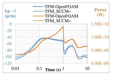
Figure 5 - Evolution of power and prompt criticality margin during 1000 pcm reactivity insertion in 1 s
