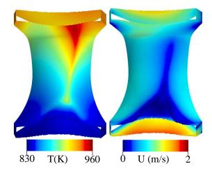
Figure 20 - Temperature and velocity distributions near the core wall for the 4 loops 1.8m<sup>3</sup> reactor
