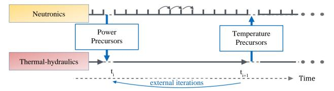
Figure 3 - Coupling scheme between neutronics and thermal-hydraulics codes [3][5]
