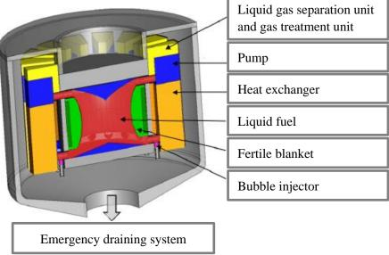
Figure 1 - Schematic view of MSFR fuel circuit [3]
