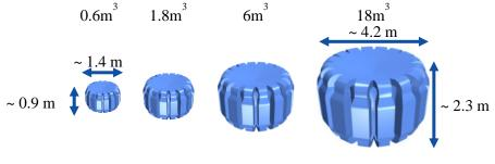
Figure 7 - Alternative versions with a total volume of 0.6 m3, 1.8 m3, 6m3 and 18m3
