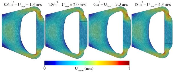
Figure 8 - Evolution of the normalized velocity for different reactor sizes and their normalization factor (maximum velocity amplitude)
