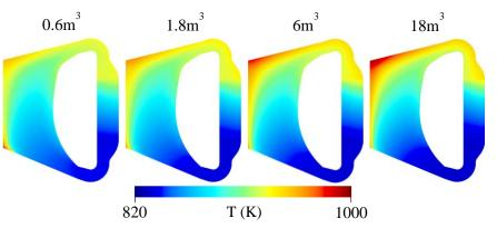
**Figure 13 - Temperature field for different reactor sizes**
