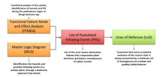
Figure 8: Complementarity between the FFMEA and the MLD methods
