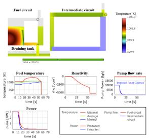
Figure 5: Loss of intermediate flow at 10s leading to an emergency draining of the fuel in the emergency draining system: view of the MSFR circuits modelled (top) and results of the calculations (bottom)
