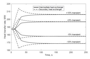
Figure 6: Evolution of the heat transfer rates in the heat exchangers for gas mass flow rate transients in the intermediate circuit
