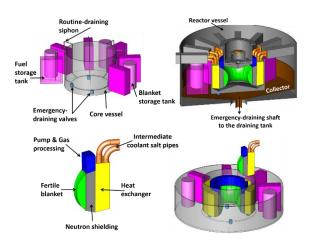
Figure 3: Schematic view of the integrated design of the MSFR fuel circuit
