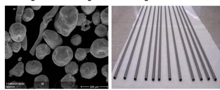
Figure 9: MA bearing fuel and cladding tube fabrication
