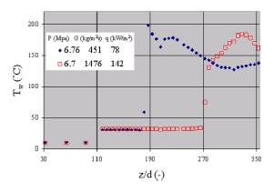
Figure 7: Wall-temperature measurements at supercritical pressures in an 8 mm tube with carbon dioxide flow
