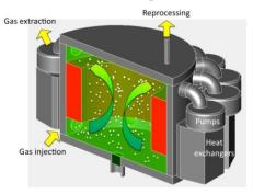
In the MSFR, the liquid fuel processing is performed on a small side stream of the molten salt. Fission products are removed from the side stream and the remainder is then returned to the reactor. This is fundamentally different from a solid fuel reactor where separate facilities produce the solid fuel and process the used nuclear fuel. Because of this design characteristic compared to classical solid-fuel reactors, the MSFR can thus operate with widely varying fuel compositions.
