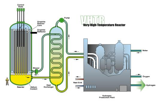
Figure 1: The VHTR for hydrogen production
