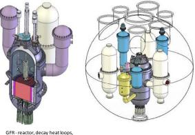
GFR - reactor, decay heat loops, main heat exchangers and fuel handling equipment
