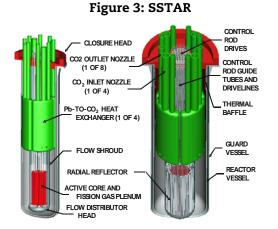
Several of the relevant characteristics of the SSTAR design are summarized in Table 3.
